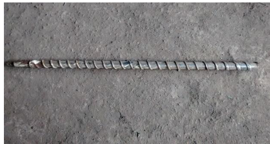
Fig.2: Photograph of failed reciprocating screw.
